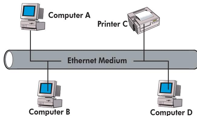
Since a signal on the Ethernet medium reaches every attached node, the destination address is critical to identify the intended recipient of the frame. For example, in the figure above, when computer B transmits to printer C, computers A and D will still receive and examine the frame. However, when a station first receives a frame, it checks the destination address to see if the frame is intended for itself. If it is not, the station discards the frame without even examining its contents.
